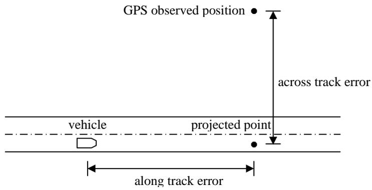
FIGURE 5: ACROSS TRACK ERROR AND ALONG TRACK ERROR
