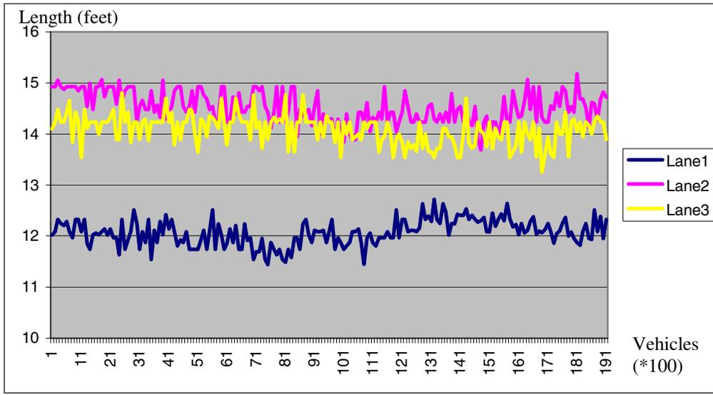
**Figure 5 - Estimated Short Vehicle Median Length at ES-167D (SB I-5 & NE 145<sup>th</sup> St.)**
