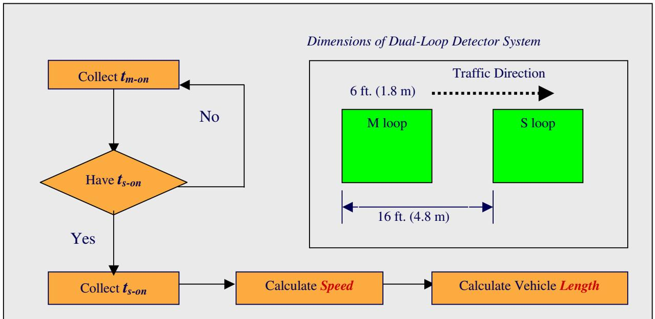
**Figure 3 - ALEDA Speed & Length Algorithm**
