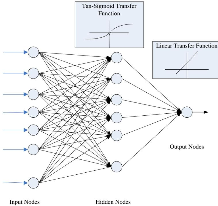
**FIGURE 1 The architecture of the proposed artificial neural network model.**
