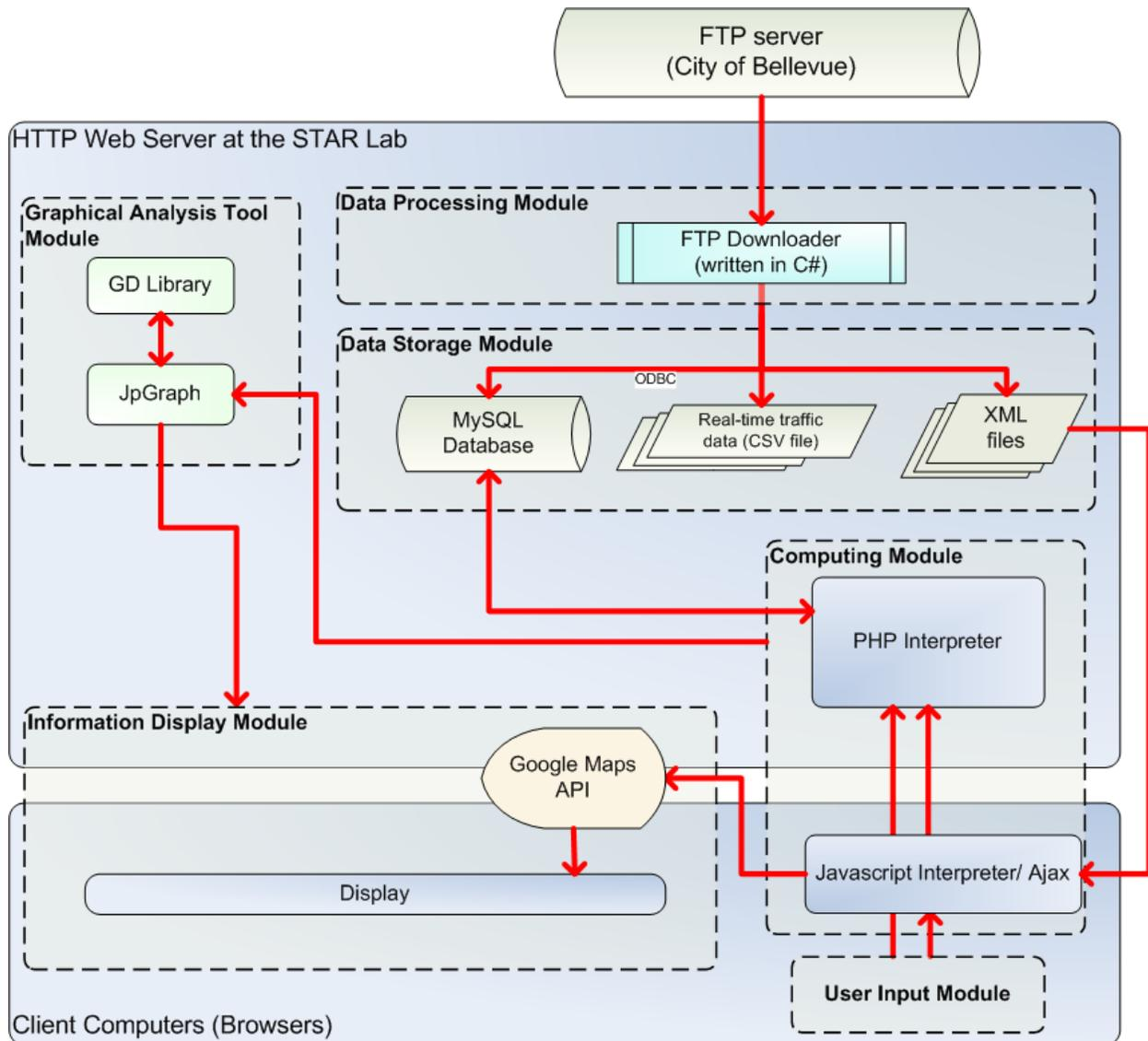
**FIGURE 3** The flow chart of the GATI system
