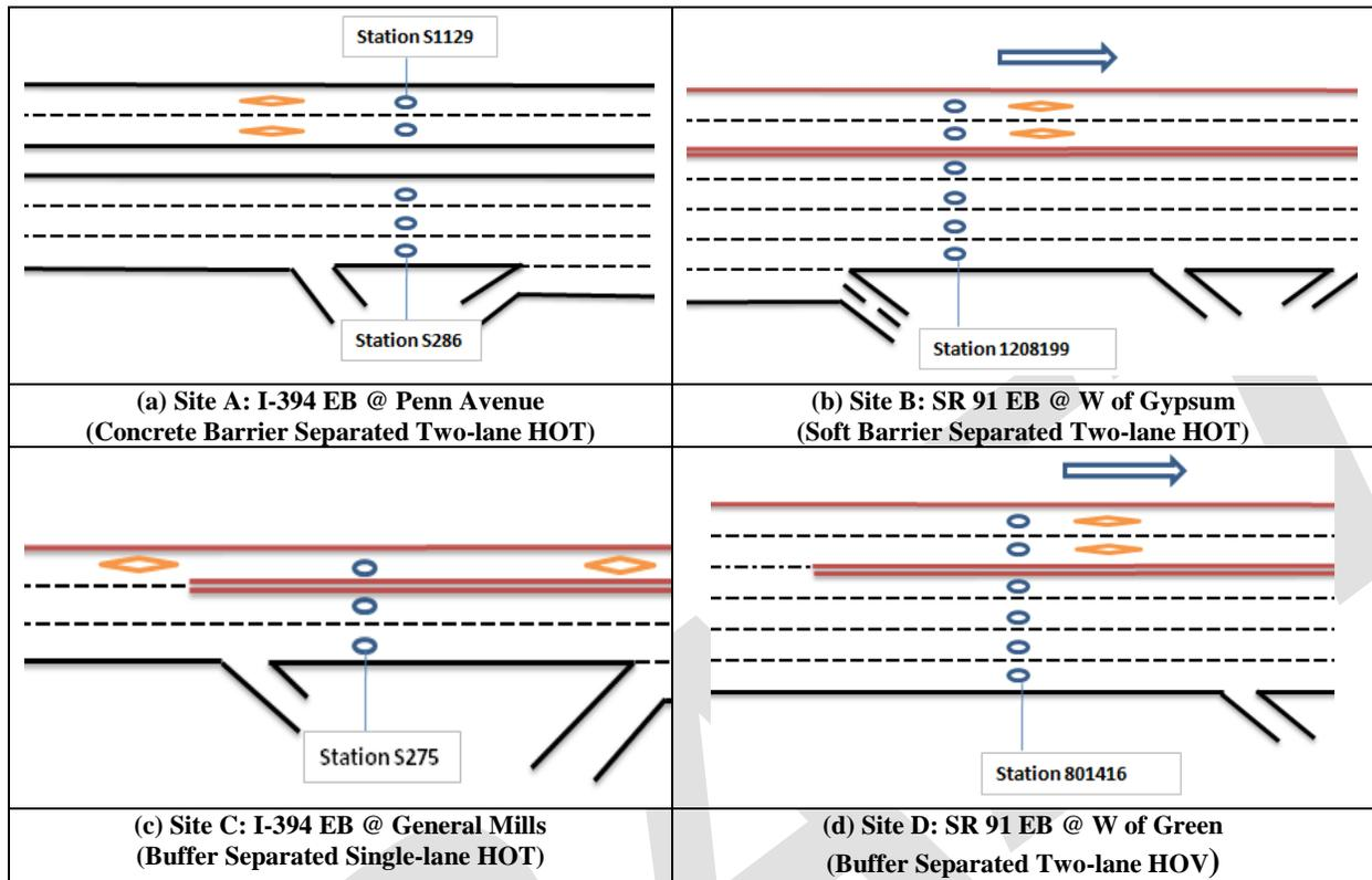
FIGURE 1 Schematics of site configurations (not to scale).
