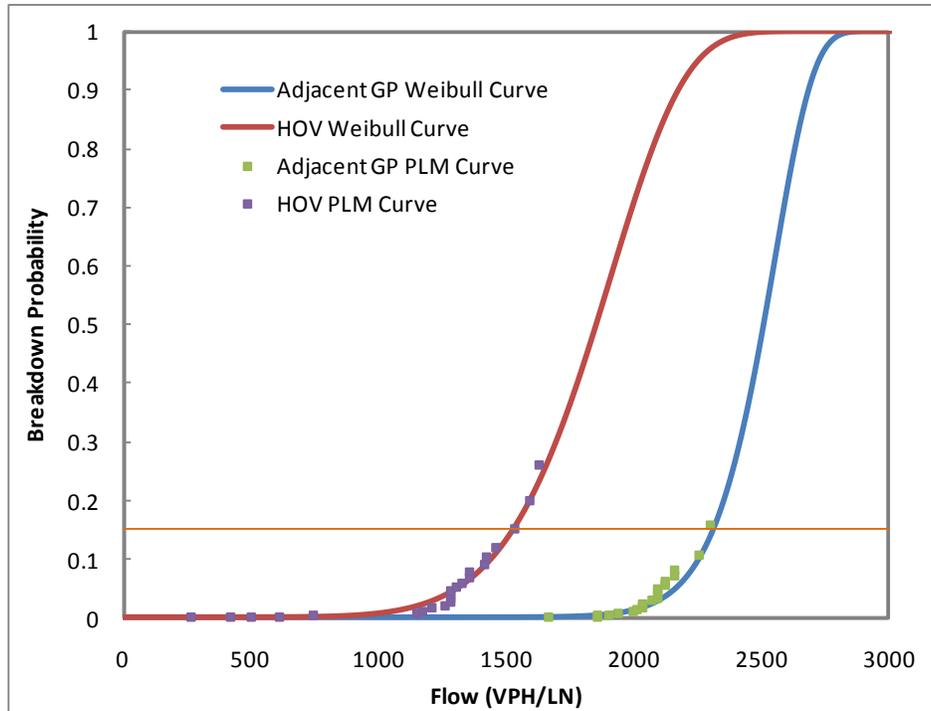
**FIGURE 8** Estimated capacity distribution functions for Site D using PLM and Weibull Method.
