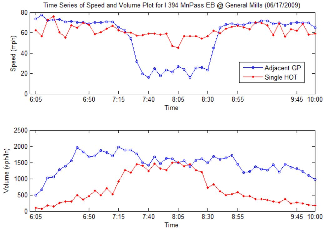
FIGURE 3 Time series of speed and flow plots for Site C.
